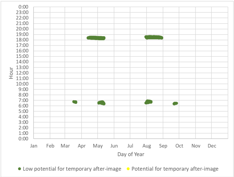
Figure 7-4 – Annual Predicted Glare occurrence with a reduced Project PV array footprint for Township Road 400 (Passenger, \pm 15^\circ FOV)
